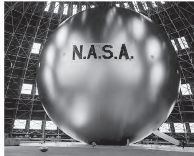
Project Echo inflation test, April 1960, Weeksville, NC.
